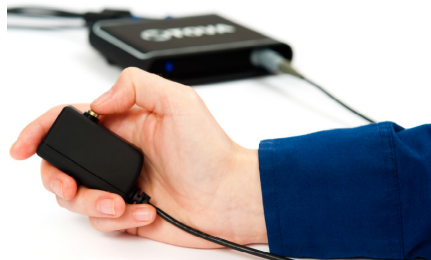
Figure 78: How to hold the microswitch
