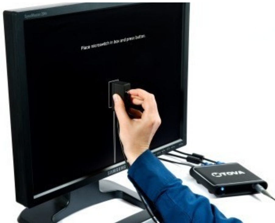
Figure 27: Calibrating the T.O.V.A. to your display.
