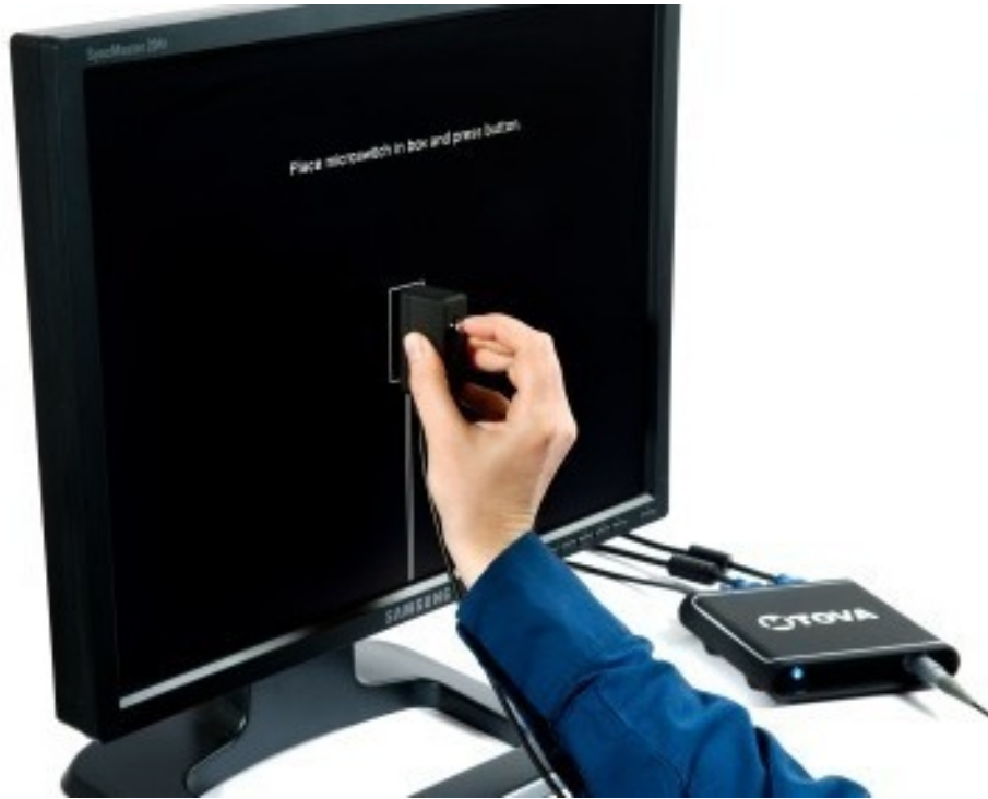
Figure 64: How to hold your microswitch for calibration
